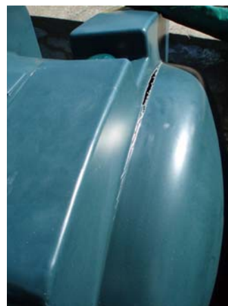
Split in a plastic tank
